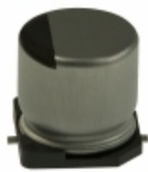
EEE-HA1V470AP Panasonic Electronic Components CAP ALUM 47UF 20% 35V SMD
