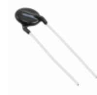
ERZ-E08A511CS Panasonic Electronic Components VARISTOR 510V 3.5KA DISC 10.5MM
