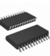
A6276SLWTR Allegro MicroSystems, LLC IC LED DRIVER LIN 75.5MA 24SOIC
