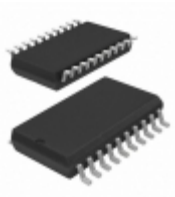
A6277SLW Allegro MicroSystems, LLC IC LED DRIVER LIN 150MA 20SOIC
