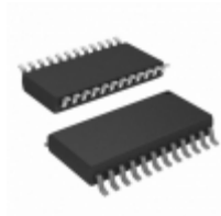
A6276SLWTR-T Allegro MicroSystems, LLC IC LED DRIVER LIN 75.5MA 24SOIC
