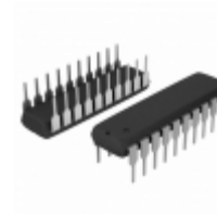
A6277EA-T Allegro MicroSystems, LLC IC LED DRIVER LINEAR 120MA 20DIP
