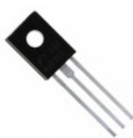
MJE170STU Fairchild/ON Semiconductor TRANS PNP 40V 3A TO-126
