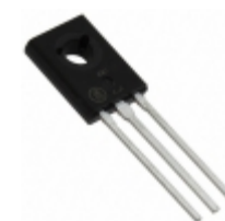
MJE171 ON Semiconductor TRANS PNP 60V 3A TO225AA
