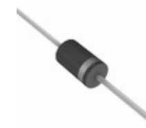
SR506 B0G TSC (Taiwan Semiconductor) DIODE SCHOTTKY 60V 5A DO201AD
