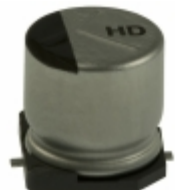
EEV-HD1C221P Panasonic Electronic Components CAP ALUM 220UF 20% 16V SMD
