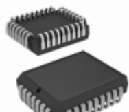
AT29LV020-12JU Microchip Technology IC FLASH 2MBIT 120NS 32PLCC
