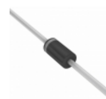
1M120ZHB0G TSC (Taiwan Semiconductor) DIODE ZENER 120V 1W DO204AL
