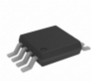
ADG723BRMZ-REEL7 Analog Devices Inc. IC SWITCH DUAL SPST 8MSOP
