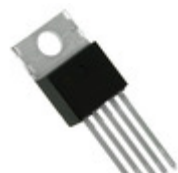
MCP1825-3302E/AT Microchip Technology IC REG LDO 3.3V 0.5A TO220-5
