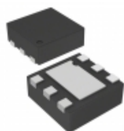
RT9081A-09GQZA(2) Richtek USA Inc. IC LDO 0.5A LOW DROPOUT ZADFN-6
