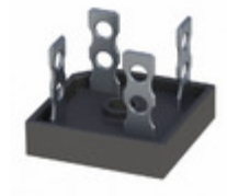
GBPC5010M T0G TSC (Taiwan Semiconductor) BRIDGE RECT 1P 1KV 50A GBPC40-M
