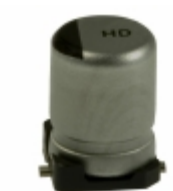
EEV-HD1H3R3R Panasonic Electronic Components CAP ALUM 3.3UF 20% 50V SMD
