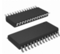
AT27BV256-15RC Microchip Technology IC OTP 256KBIT 150NS 28SOIC
