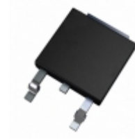
IRFR3711TR Infineon Technologies MOSFET N-CH 20V 100A DPAK
