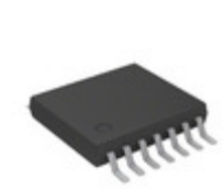
MCP6H74-E/ST Microchip Technology IC OPAMP GP 2.7MHZ RRO 14TSSOP
