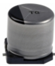
EEE-TG1C221P Panasonic Electronic Components CAP ALUM 220UF 20% 16V SMD
