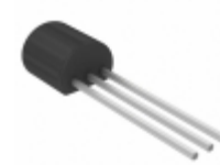
MIC5207-3.3BZ Microchip Technology IC REG LDO 3.3V 0.18A TO92-3
