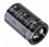
LGY1H562MELA40 Nichicon CAP ALUM 5600UF 20% 50V SNAP
