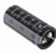
LGY1H562MELZ50 Nichicon CAP ALUM 5600UF 20% 50V SNAP
