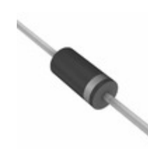
BZW06-26 B0G TSC (Taiwan Semiconductor) TVS DIODE 25.6V 53.5V DO204AC
