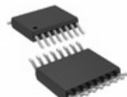
LTC2367IMS-18#PBF ADI (Analog Devices, Inc.) IC ADC 18BIT 500K 1CH 16MSOP
