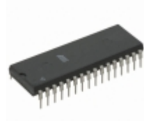
AT28LV010-20PI Microchip Technology IC EEPROM 1MBIT 200NS 32DIP
