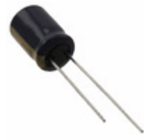
EEU-FC1E221B Panasonic Electronic Components CAP ALUM 220UF 20% 25V RADIAL
