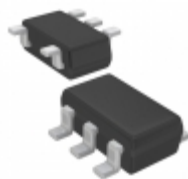
XC6124C629MR-G Torex Semiconductor Ltd IC WATCHDOG TIMER SOT-25
