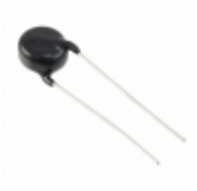
ERZ-E10A751 Panasonic Electronic Components VARISTOR 750V 4.5KA DISC 12.50MM
