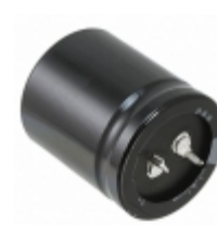
LGR2D681MELB35 Nichicon CAP ALUM 680UF 20% 200V SNAP
