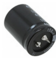
LGR2D821MELB40 Nichicon CAP ALUM 820UF 20% 200V SNAP
