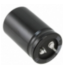
LGR2D681MELA40 Nichicon CAP ALUM 680UF 20% 200V SNAP
