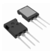
IXGX72N60B3H1 IXYS IGBT 600V 75A 540W PLUS247
