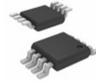
SY10EL16VBKG TR Microchip Technology IC RCVR DIFF 3.3/5V 8MSOP
