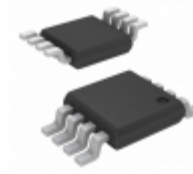
S-1410I45-K8T2U4 SII Semiconductor Corporation TIMER WITH RESET FUNCTION
