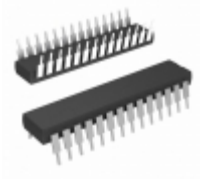
PIC16C73A-20E/SP Microchip Technology IC MCU 8BIT 7KB OTP 28SDIP
