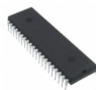
TS87C51RD2-MIA Microchip Technology IC MCU 8BIT 64KB OTP 40PDIL
