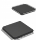
CS8952-CQ Cirrus Logic Inc. IC ETHNT 10/100 TXRX 5V 100-TQFP
