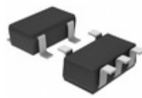
BD4730G-TR Rohm Semiconductor IC RESET CPU BIPOLAR 3.0V 5SSOP
