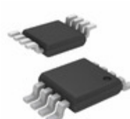
MIC7300YMM Microchip Technology IC OPAMP GP 370KHZ RRO 8MSOP
