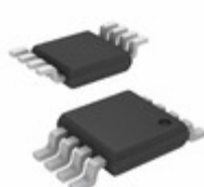
MIC7300BMM-TR Microchip Technology IC OPAMP GP 370KHZ RRO 8MSOP
