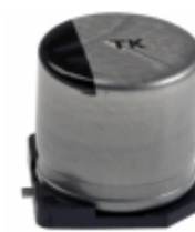
EEE-TK1A222AM Panasonic Electronic Components CAP ALUM 2200UF 20% 10V SMD
