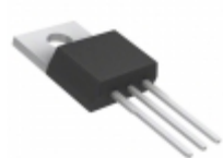
KA7918TU Fairchild/ON Semiconductor IC REG LDO -18V 1A TO220-3
