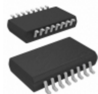
ADUM4400WBRWZ ADI (Analog Devices, Inc.) DGTL ISO 5KV 4CH GEN PURP 16SOIC
