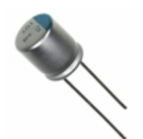
APSC100ELL681MJB5S United Chemi-Con CAP ALUM POLY 680UF 20% 10V T/H
