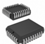
AT28C256-20JC Micrel / Microchip Technology IC EEPROM 256KBIT 200NS 32PLCC
