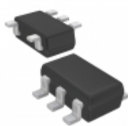
XC6123D436MR-G Torex Semiconductor Ltd IC WATCHDOG TIMER SOT-25
