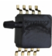
MPXAZ6115APT1 NXP USA Inc. SENSOR PRESSURE ABSOLUTE 8-SOP
