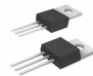
IXTP16N50P IXYS MOSFET N-CH 500V 16A TO-220
