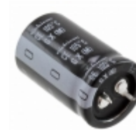
LGX2G271MELA40 Nichicon CAP ALUM 270UF 20% 400V SNAP
