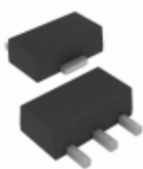
MCP1700T-2402E/MB Microchip Technology IC REG LDO 2.4V 0.2A SOT89-3
