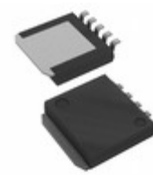
BD3572YHFP-MTR LAPIS Semiconductor IC REG LINEAR POS ADJ 500MA HRP5
