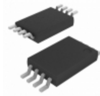
BA4558FV-E2 Rohm Semiconductor IC OPAMP GP LN 2MHZ 8SSOP
