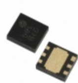
XC6121D542ER-G Torex Semiconductor Ltd IC WATCHDOG TIMER 6-USP
