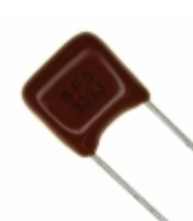
ECQ-B1H333JF Panasonic Electronic Components CAP FILM 0.033UF 5% 50VDC RADIAL
