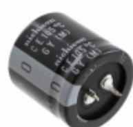
LGY2W121MELB Nichicon CAP ALUM 120UF 20% 450V SNAP
