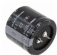
LGY2W151MELC Nichicon CAP ALUM 150UF 20% 450V SNAP
