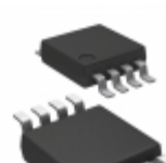
24LC64FT-E/MS Microchip Technology IC EEPROM 64KBIT 400KHZ 8MSOP
